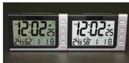
Reflective LCD using LINTEC's light diffusion film (right)
