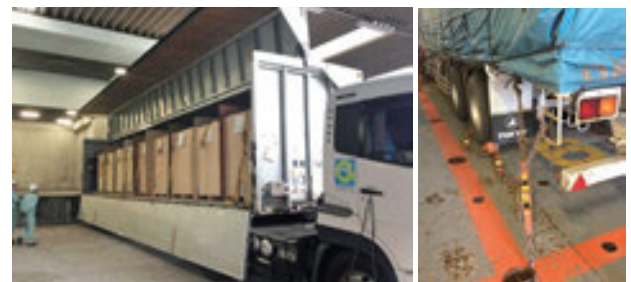
Securing goods in the cargo area of the truck to prevent them from collapsing (left) and securing the truck on the ship (right)
