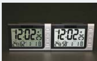
Reflective LCD using LINTEC’s light diffusion film (right)
