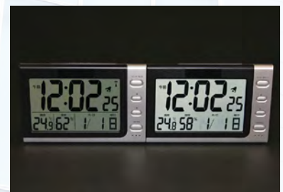
Reflective LCD using LINTEC's light diffusion film (right)
