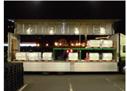
Double-deck structure introduced in 10-ton trucks to improve loading efficiency
